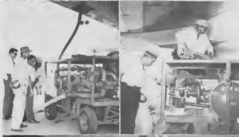
HYDRANT CARTS used in fastening deliver 17,000 gallons an hour.
